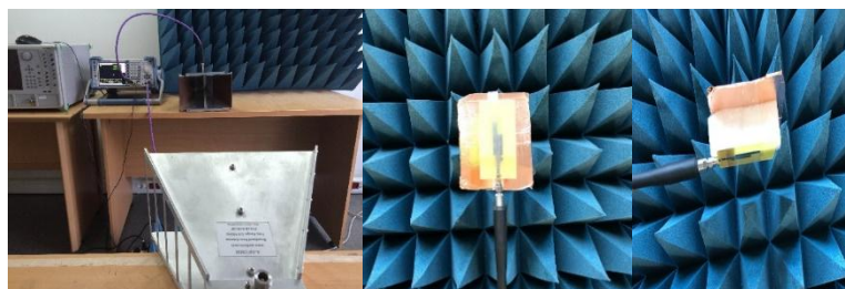
Fig. 7 Measurement Setup for Maximum Far Field Gain.
